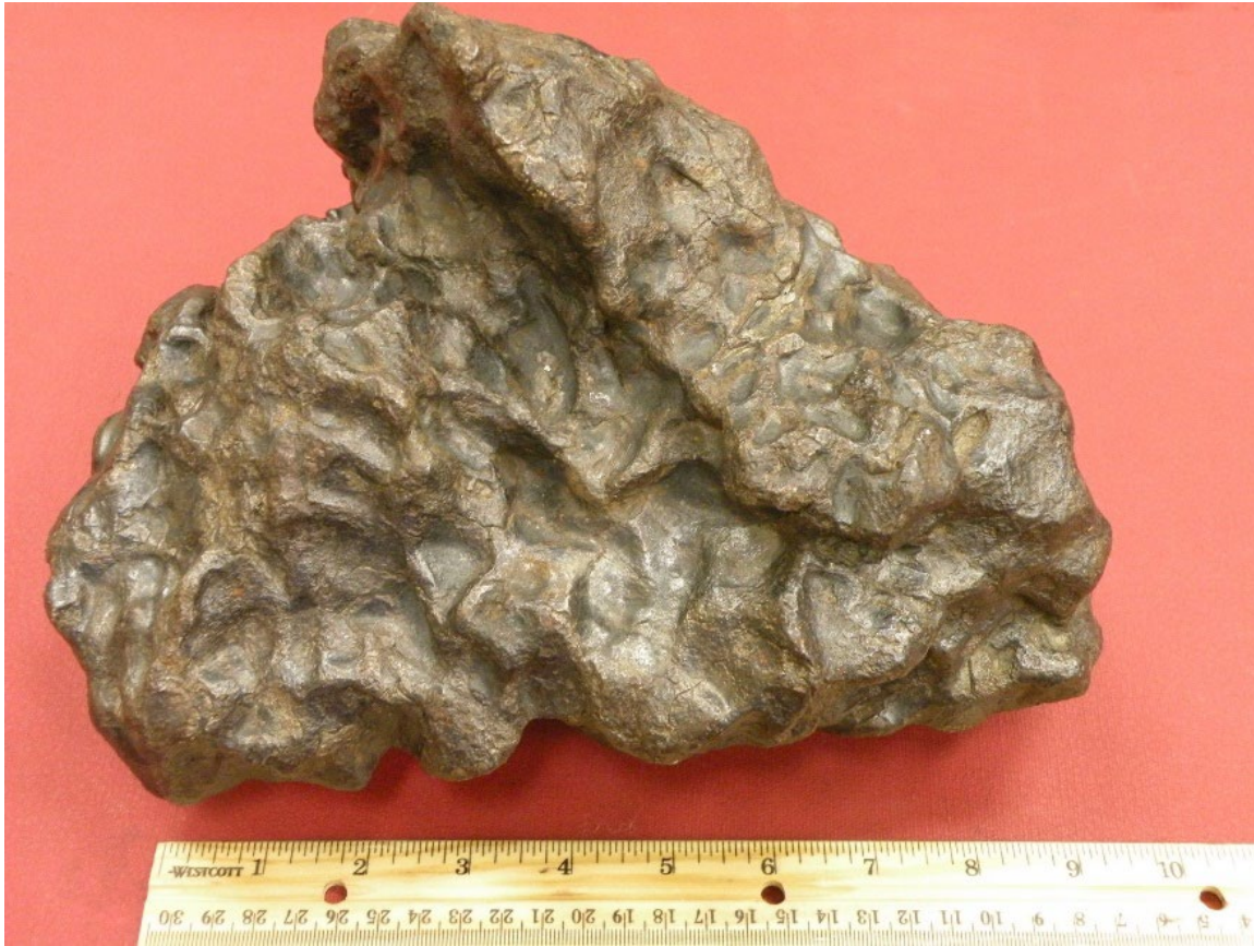
Figure 2 - Iron meteorite from Russia with "thumb print"-like regmaglypts on the outer surface (magnetic). From University of Arkansas, Little Rock, collection.
