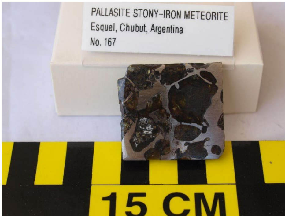
Figure 9 – Pallasite, a type of stony-iron meteorite, from Argentina that contains crystals of olivine in iron-nickel matrix (magnetic). From the author's collection.
