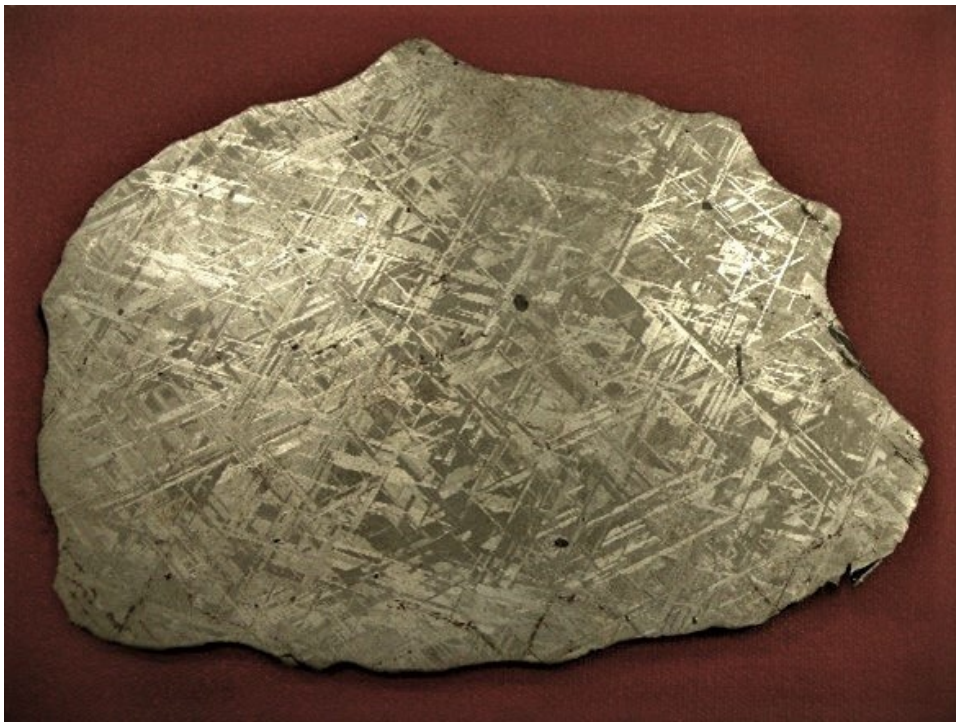
Figure 7 - Iron meteorite with Widmanstätten (crystal structure) pattern. From University of Arkansas, Little Rock, collection.
