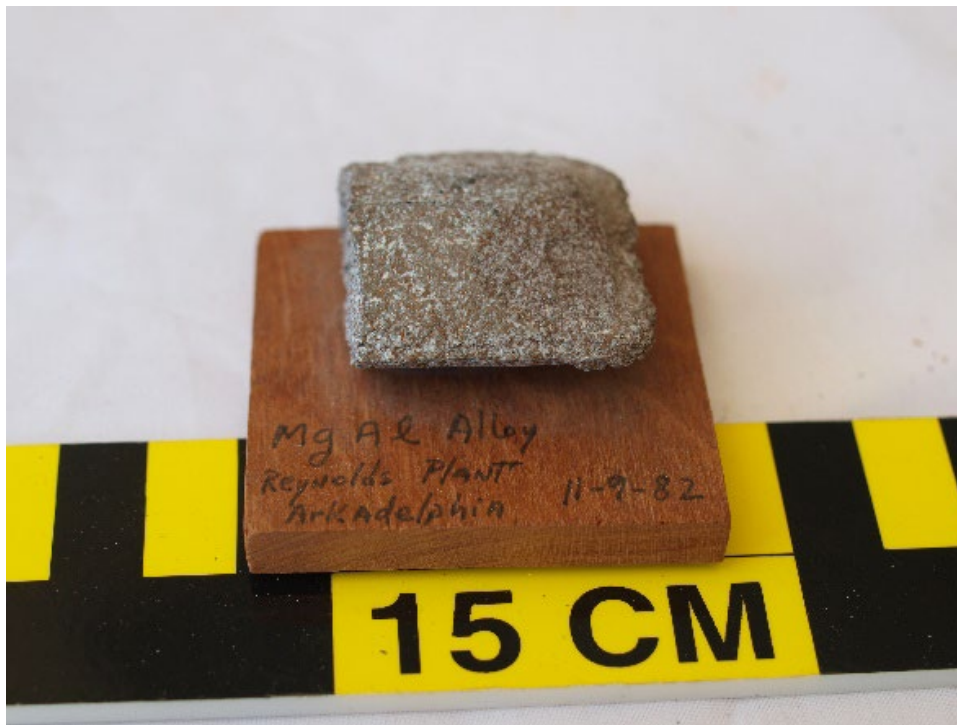
Figure 27 - Magnesium aluminum iron alloy that was created as a waste material of aluminum production in Arkansas (magnetic).
