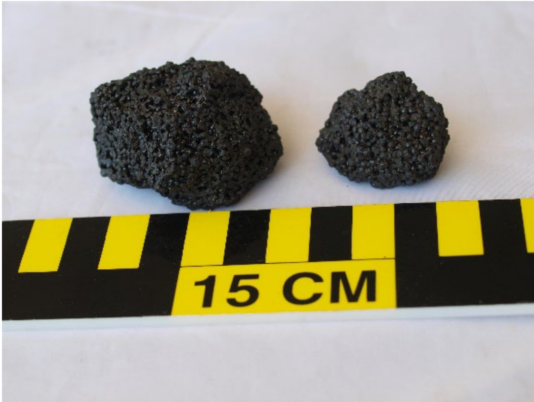
Figure 34 - Vuggy, glassy clinker (non-magnetic). A vug is a cavity or large pore in a rock or man-made material.
